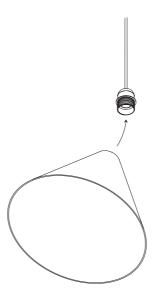
Place the plastic shade support on the bulb holder and replace the lower shade ring to fix it in place. The plastic conical insert that the shade support connects with stops the shade from being dislodged during use for e.g. cleaning.
