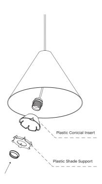
Place the shade over the bulb holder, ensuring it is parallel to the floor.
